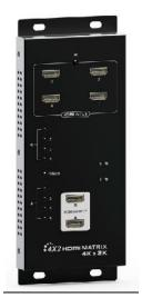
This 4x2 HDMI Matrix Switch is with 4 HDMI inputs and 2 HDMI outputs. It is a true matrix and can distribute any one of 4 sources to either of 2 displays, and can work as a splitter to show the same source on 2 displays simultaneously. Analog R/L audio and digital SPDIF audio can be extracted from HDMI signal. It supports 3D HDMI and HDMI1.4 (4kx2K).
